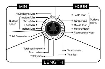
3. After attaching proper adapter or wheel, bring it into contact with rotating object moving surface whose speed is to be measured.
