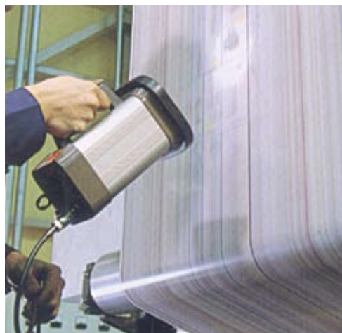
Printing Inspection: Color Registration
