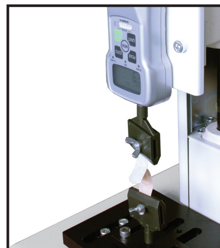
Stand with Optional Grip Performing Peel Test
