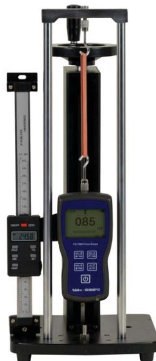
FGS-250W with FG-7000 Force Gauge Shown Performing Tensile Test
